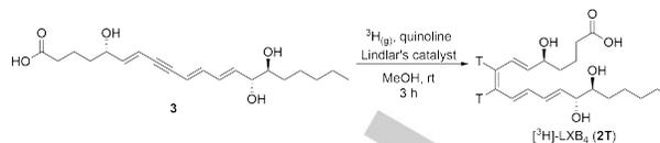
**Scheme 5.** Synthesis of tritiated LXB<sub>4</sub> (**2T**) via hydrogenation with Lindlar's catalyst and tritium gas.
